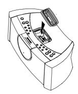
3.) Mount the iPod® Support Bracket on the docking station as shown. This bracket provides support and prevents your iPod® from moving too far backward when you operate the iPod® controls.
